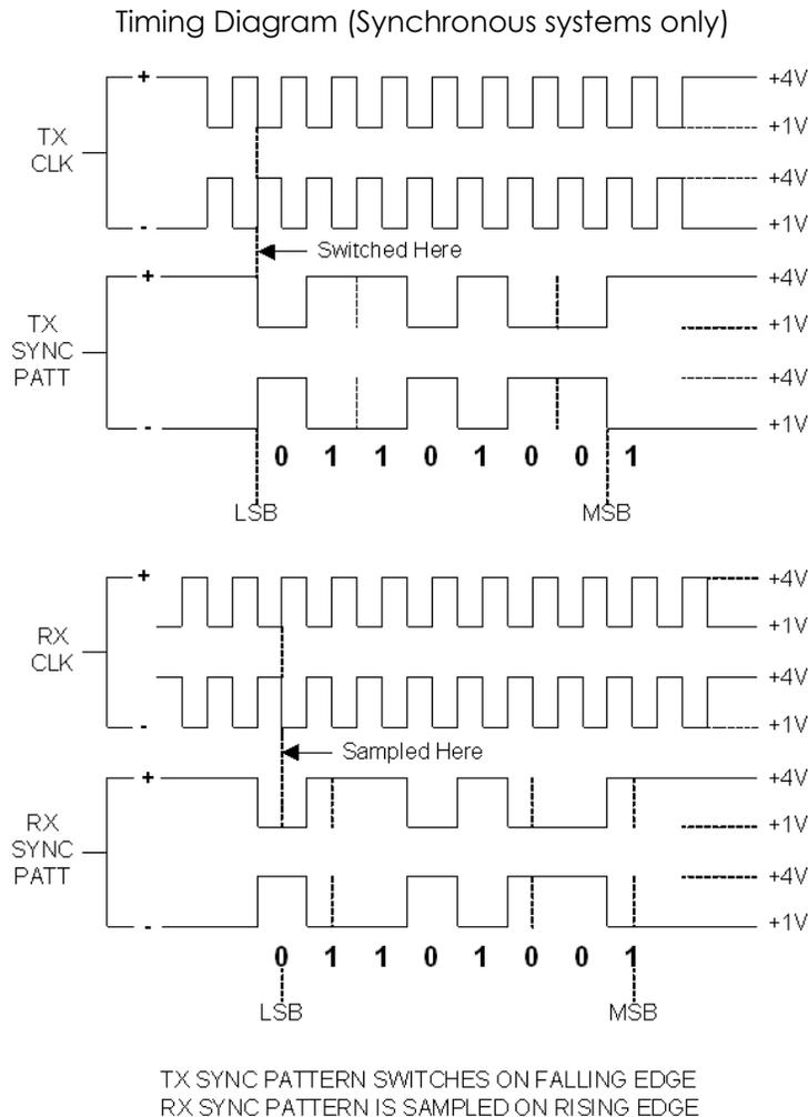
**Troubleshooting Procedures** (cont.)**Digital RS-422 Ports – Advanced Diagnostics Using Oscilloscope** (cont.)
