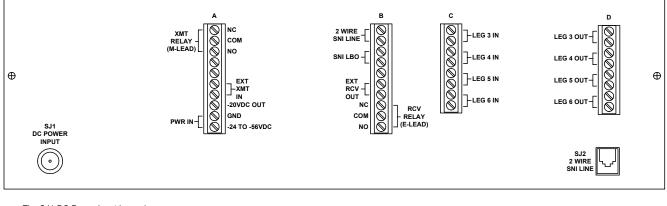
The SJ1 DC Power Input is used with an optional AC Power Pack.
