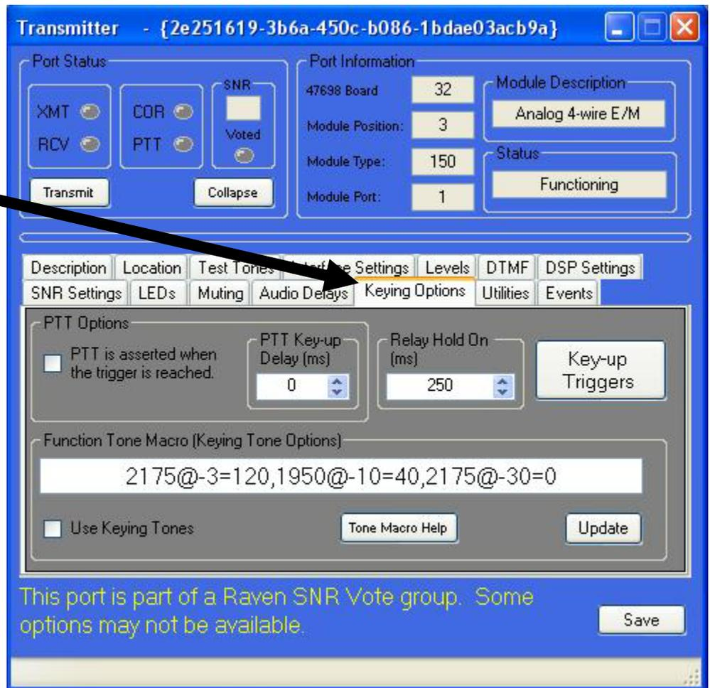
A transmitter can be optionally keyed using either PTT or keying tones. This section describes the different keying options.
