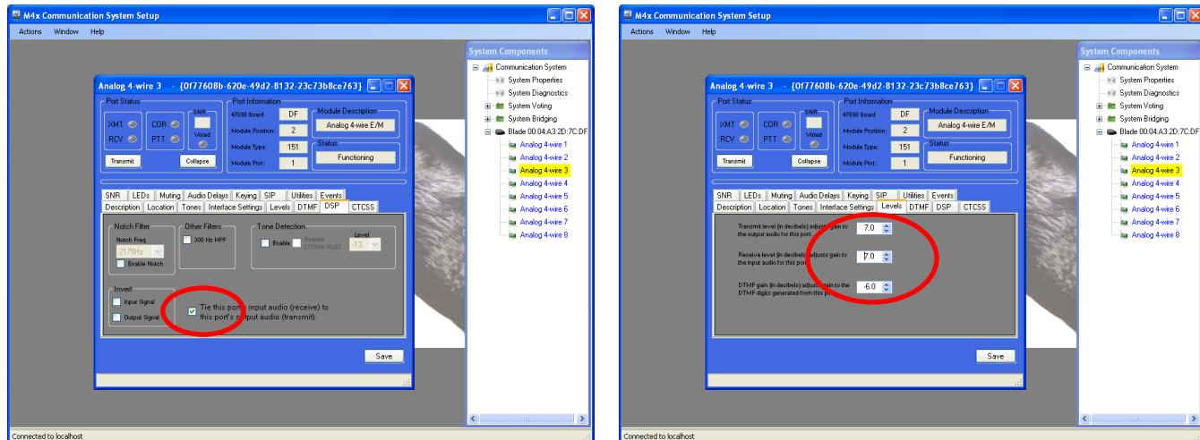
Using the prior example of a cross patch from port 1 to port 2, assume it is not desirable to add gain to the output side port 2 as shown in figure 2. Instead, port 3 configured as shown above, can be used as a *preamp port* with gain added to the input, output, or both sides of this port and then cross cabled to port 1. Port 2 can then be set back to the default output level of 0 dB or other gain or loss value.
