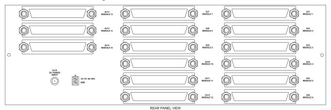
41000-204 Bridge/Hybrid/Notch Filter Shelf (Rear View)
