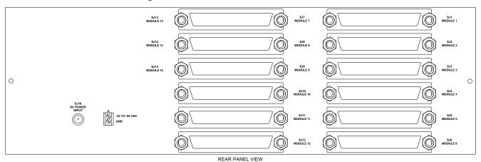
41000-224 Bridge/Hybrid/Notch Filter Shelf with Redundant Power Supplies
